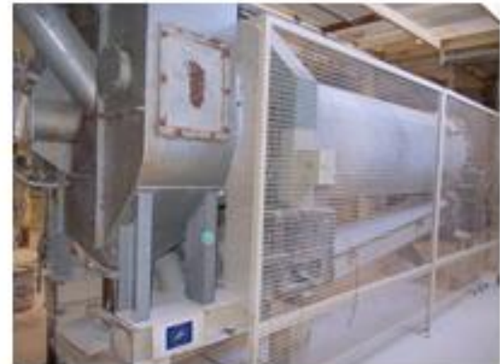
Drier with connection to the improved de-dusting system
