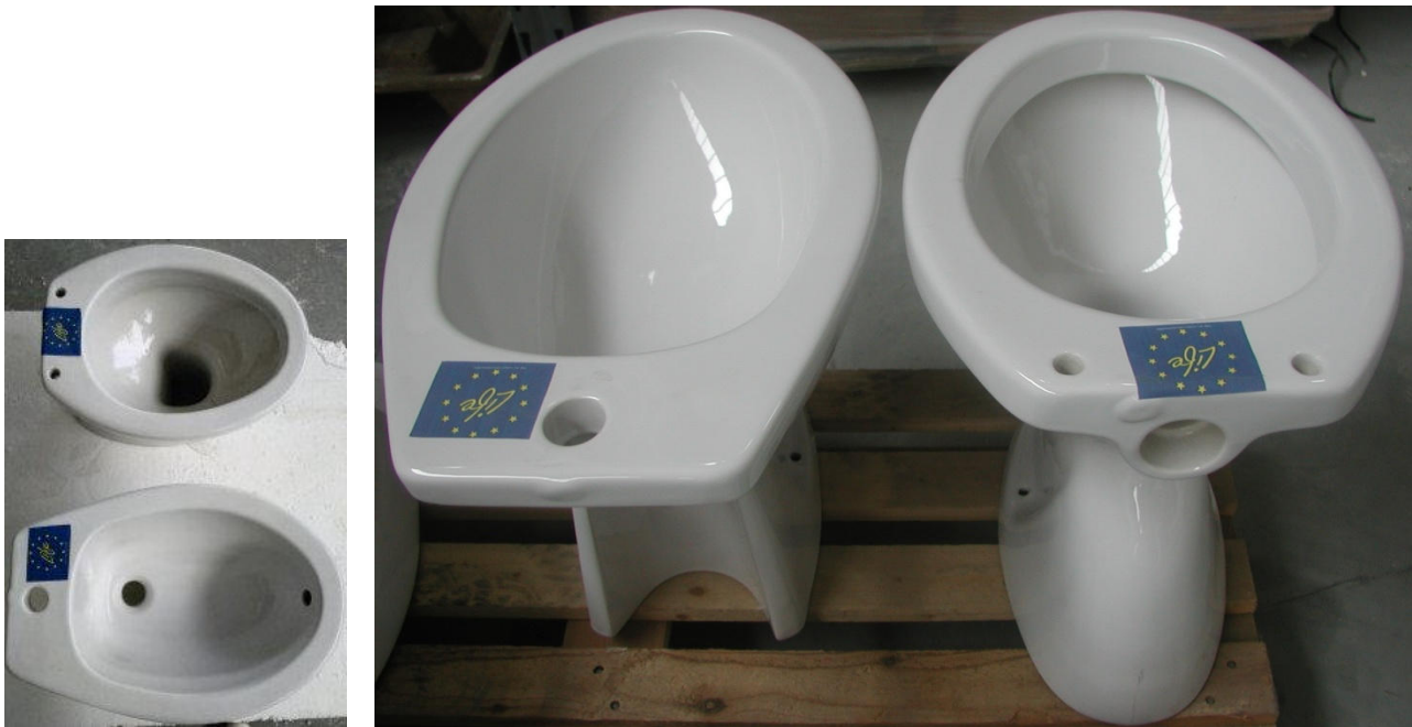
Figure 3 – Pieces made with SANITSER 13 and glaze PSI-109
