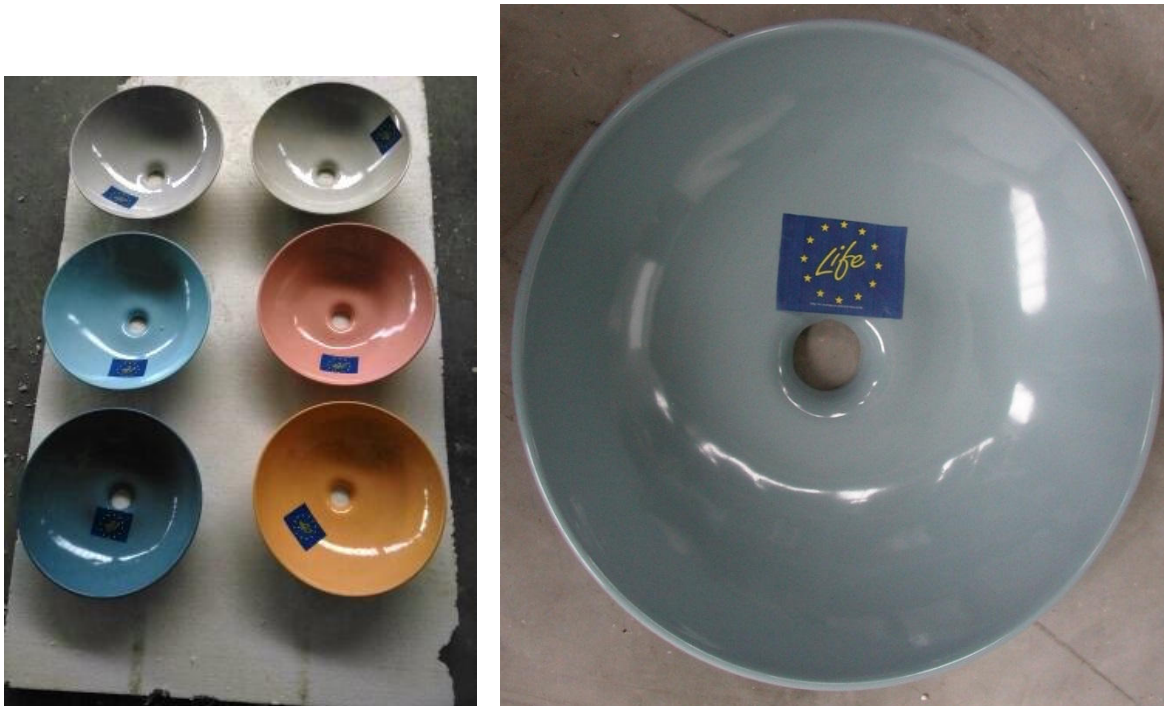
Figure 2 – Washbasins produced using slip SANITSER 13 and coloured glaze PSI-109
