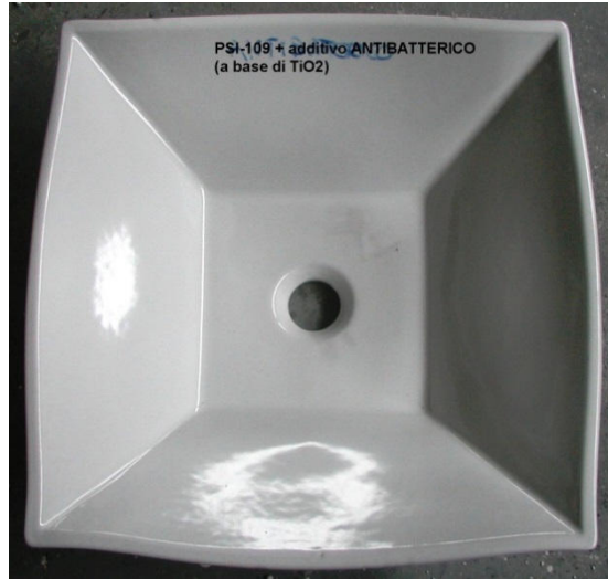
Figure 1 – Washbasin produced using slip SANITSER 13 and glaze PSI-109 with anti-bacterial additive
