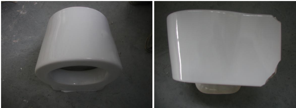
Glaze tests with two different formulations of glazes studied by GEMICA.
