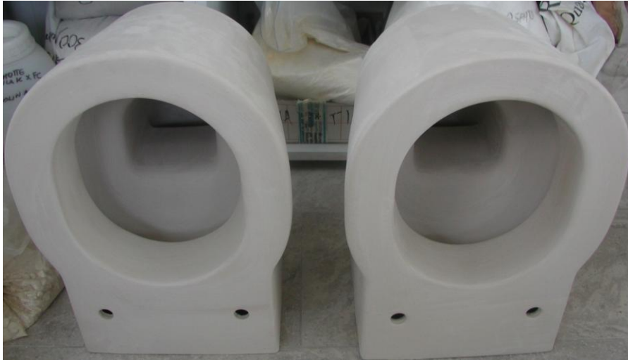
Body used for manual casting of a wc in semi-industrial test.
